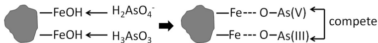
Fig. 6 A schematic of the mechanism depicting the competition between As(III) and As(V) for ferrihydrite surface sites
